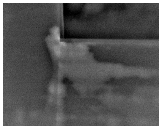
Figure 3: Convection heat loss at wall corner/flat roof perimeter detail. Masonry brick wall appears to be wet, due to moist warm air ex-filtrating through exterior wall system.
